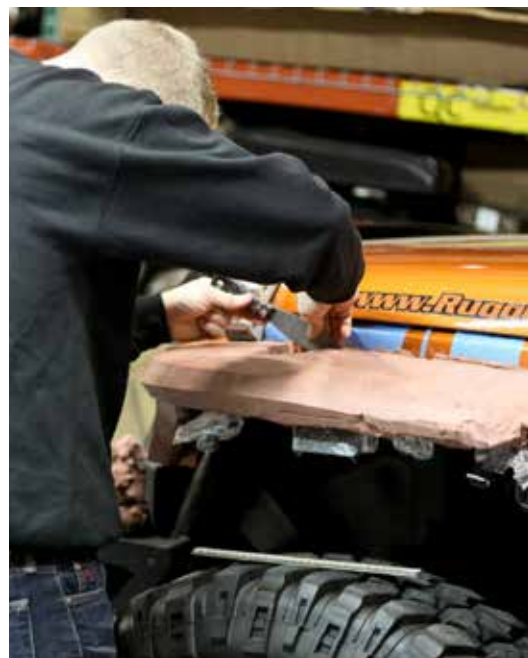
The process continues using clay, hand modeled directly on the body.
