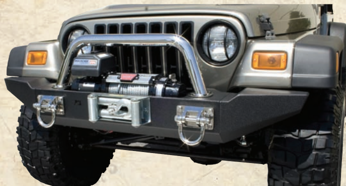
Standard Front Winch Mount With Stainless D-rings & Stainless Override Hoop: 11540.40, 11540.16, 11540.17, 11540.42
